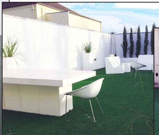
Micro-Mesh® grating and pedestals create a level, elevated rooftop terrace that ensures corrosion resistance and proper drainage. The grating surface was covered by artificial turf and outdoor furnishings, increasing the owners' living space while providing low maintenance landscaping.
